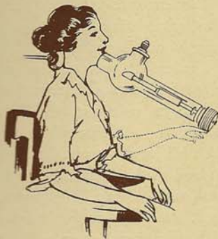
Note how the patient might raise the hand to contact with 43,000 volts from a tube with an unguarded radiator.
