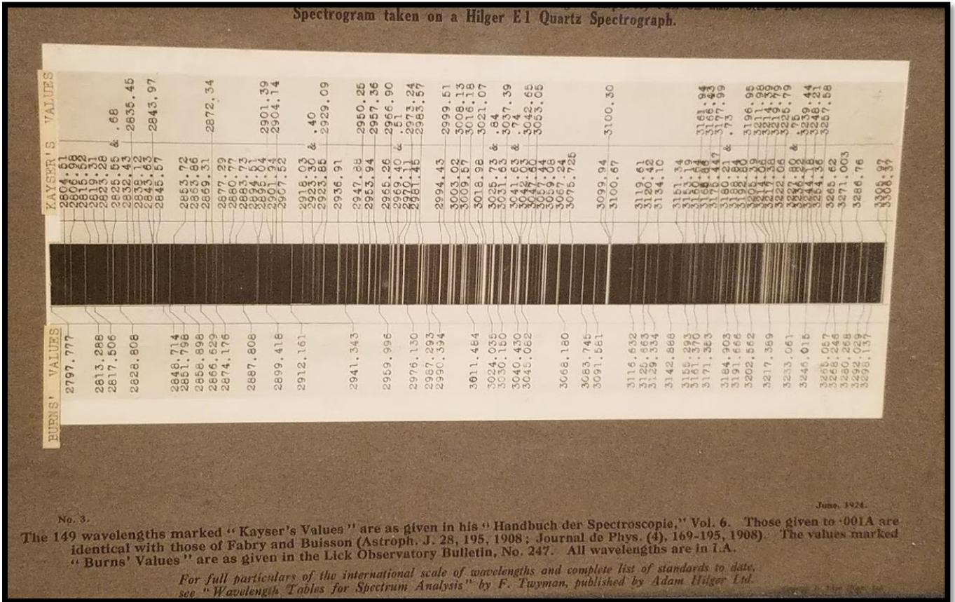
Original Spectrogram for Iron Arc Spectrum (Early 1900s, Bang lamp)
