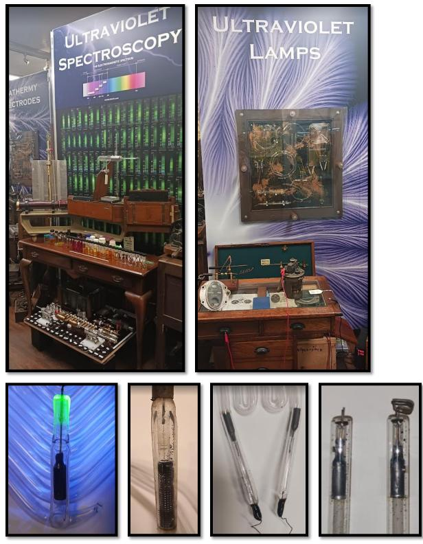
Left: Adam Hilger Spectroscope and Author's patent model Broadband Ultraviolet Sources. Right: Some of the earliest-known experimental ultraviolet lamps having a variety of unique seals and construction methods. Below: Various obscure seals in early lamps.
