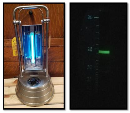
Sunkraft Cold-Quartz Ultra-Violet and Ozone Apparatus, electrodeless lamp, (1920s)
