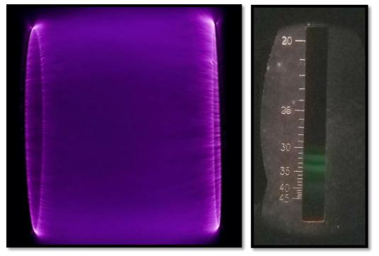
Corona Discharge from Tesla Apparatus (1892) (Replica built by author.)
